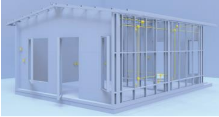
Figure 8. Window openings & building utilities
